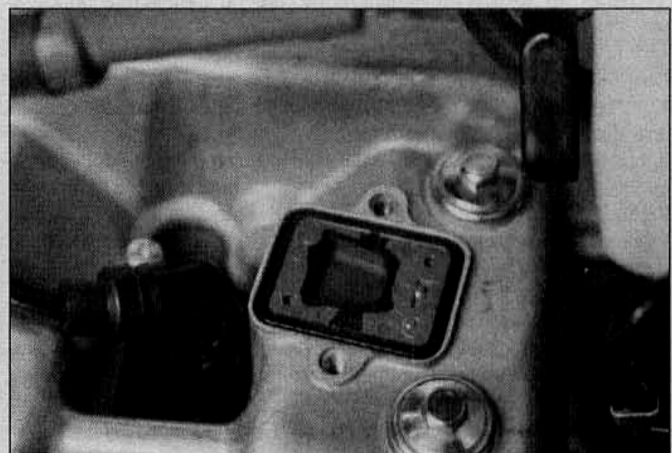
23.3b Unbolt the air suction valve from the valve cover to inspect it
