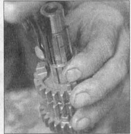
30.4f . . .then remove the snap-ring . . .
