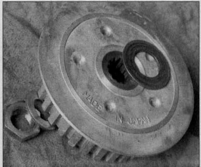
19.9a Remove the nut and washer, then remove the clutch hub and thrust washer
