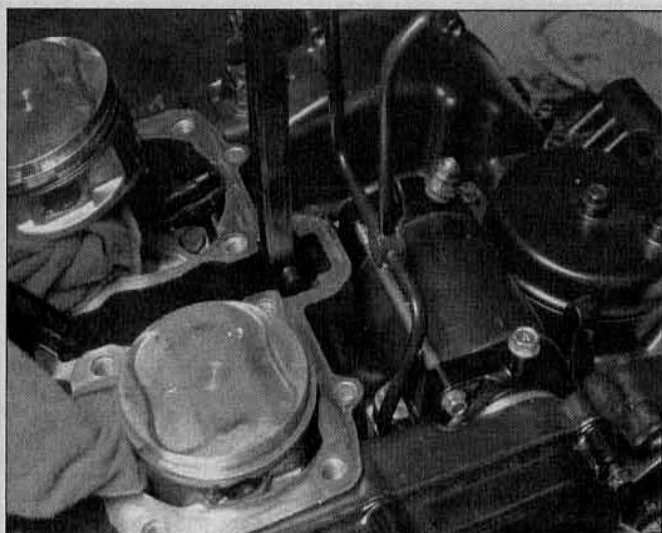
13.4 Lift the rear cam chain guide out of the engine (cylinder block removed for clarity)
