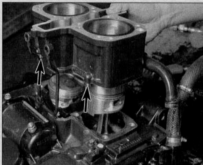
13.5 Lift the cylinder block up and off the crankcase and pistons; don't lose the dowels (arrows)
