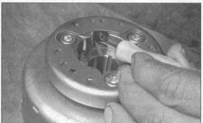
35.4a Compress the springs with a small screwdriver and remove the rollers
