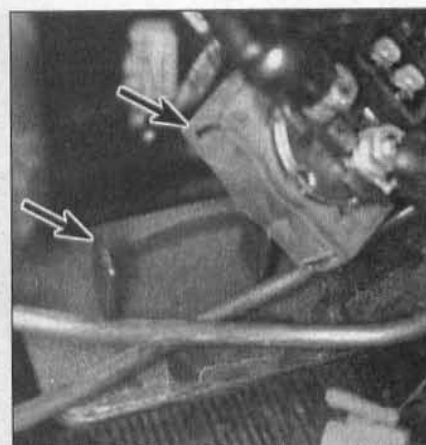
25.9 The mounting tabs fit into slots in the relay holder (arrows) - EN500 models
