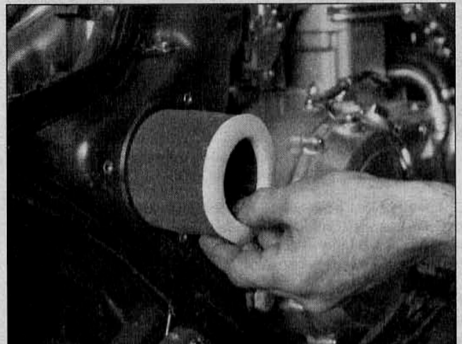
13.8b . . . and pull out the filter element
