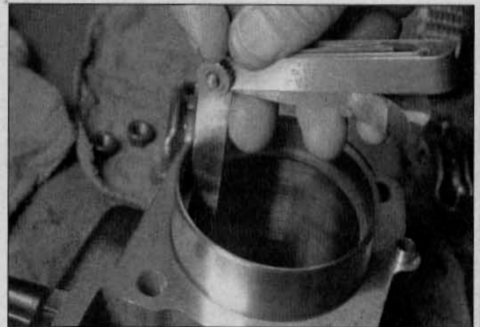
15.3b . . .then check the piston ring end gap with a feeler gauge
