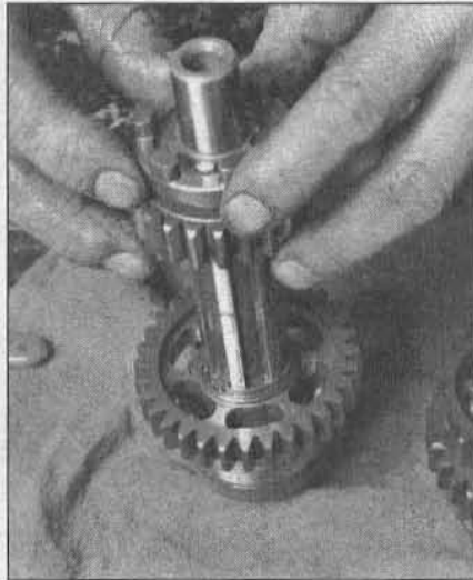
30.15k ...and slide sixth gear off the shaft
