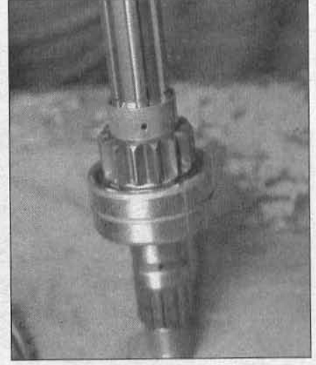
30.4j ...and the fifth gear bushing (if equipped)
