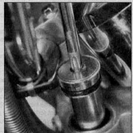
29.2c . . . once the retaining ring is removed, release the spring pressure
