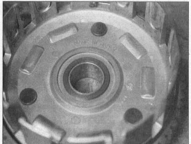
25.8 Inspect the bearing in the center of the clutch housing - replace the clutch housing if it's worn or damaged
