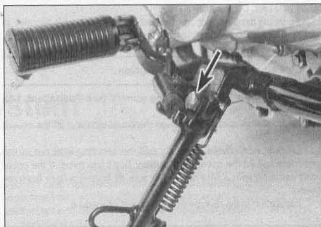
4.3 With the motorcycle securely supported, unhook the spring and remove the pivot bolt (arrow) to detach the sidestand
