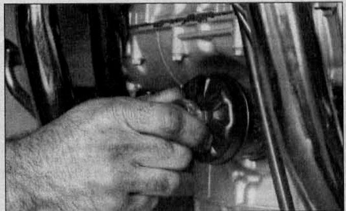
12.5a Remove the oil filter with a filter wrench or a special socket; the special socket is best, since it allows the filter to be tightened accurately with a torque wrench
