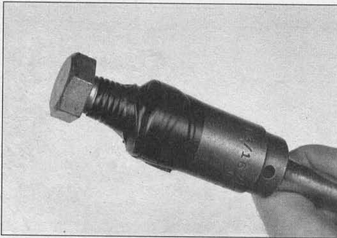
4.4d . . . then install the nut-end into a socket (connected to a long extension) and tape it into place
