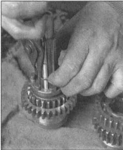
30.15j Remove the toothed washer, then the snap-ring...
