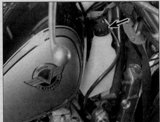
3.16 The reservoir is located inside the right side cover; to add coolant, remove the filler cap (arrow)
