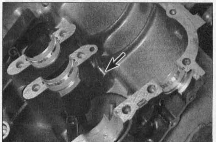
23.6b . . .after removing the crankshaft, pull out the retaining pin and remove the cam chain guide
