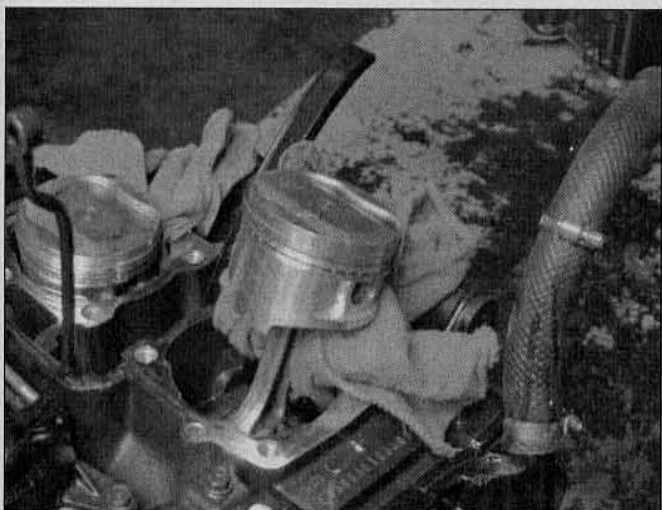
13.6 Place rags under the pistons to protect them and keep debris out of the crankcase
