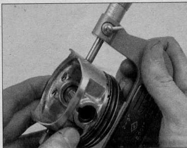
14.14a Measure the piston diameter with a micrometer
