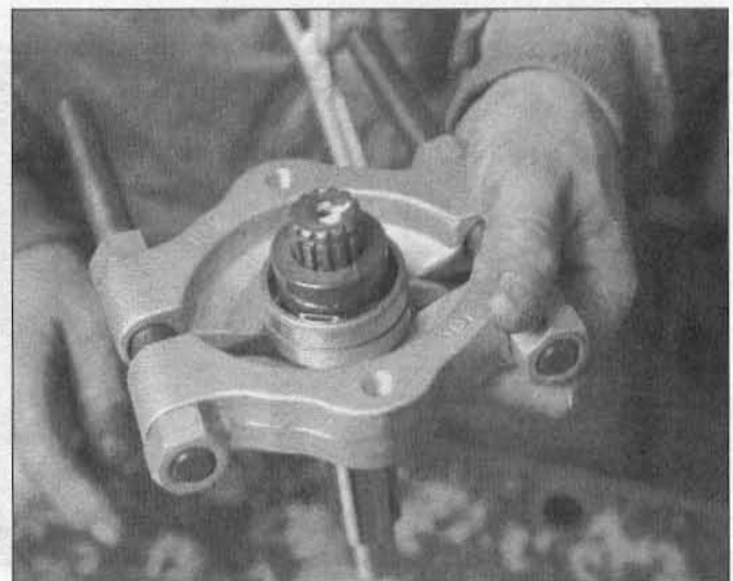
30.15p If the bearing is worn or damaged, place it in a bearing splitter, press it off the shaft and press a new one on (or have the job done by a motorcycle dealer)
