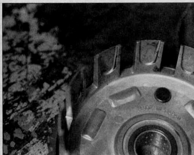
19.15 Check the slots on the clutch housing for indentations - if they're worn, the crankcase will have to be disassembled to remove the clutch housing
