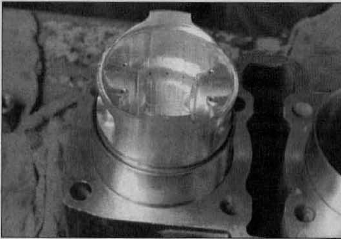
15.3a Square the ring in the bore by turning the piston upside down and tapping on the ring. . .
