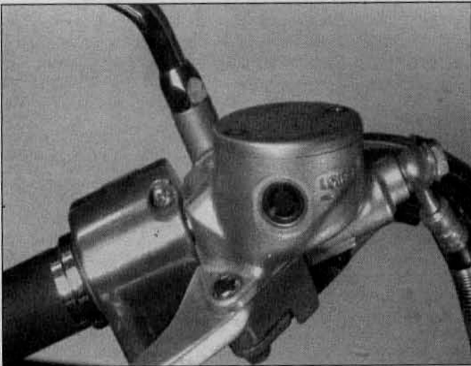
3.7 With the master cylinder in a level position, check the fluid level in the inspection window
