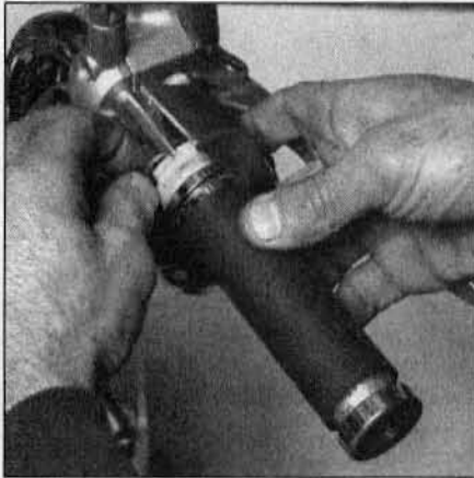
9.5a Lift the inner decelerator cable out of its groove, align it with the slots in the throttle pulley and slip the cable end out of the pulley . . .
