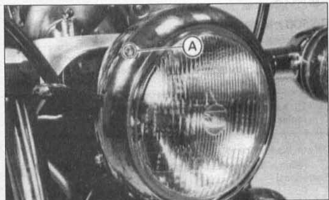
10.3b . . . and on EN500 models it's high on the right side of the headlight ring
