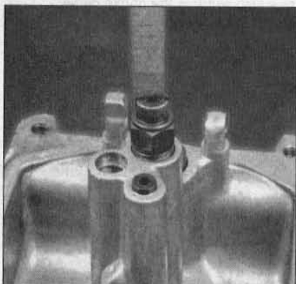
7.8 Unscrew the main jet from the needle jet holder
