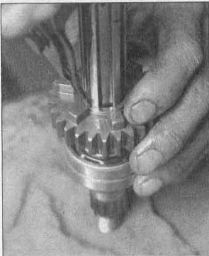
30.4h ...remove the snap-ring and toothed washer...
