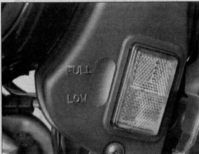
3.15 Check coolant level through the inspection hole in the right side cover; it should be between the Full and Low marks with the engine cold
