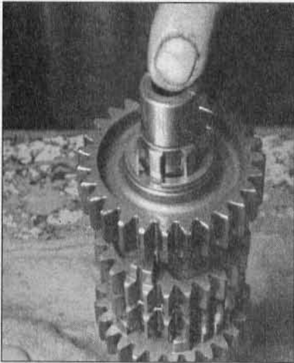
30.11h ...then secure the gear and washer with a snap-ring
