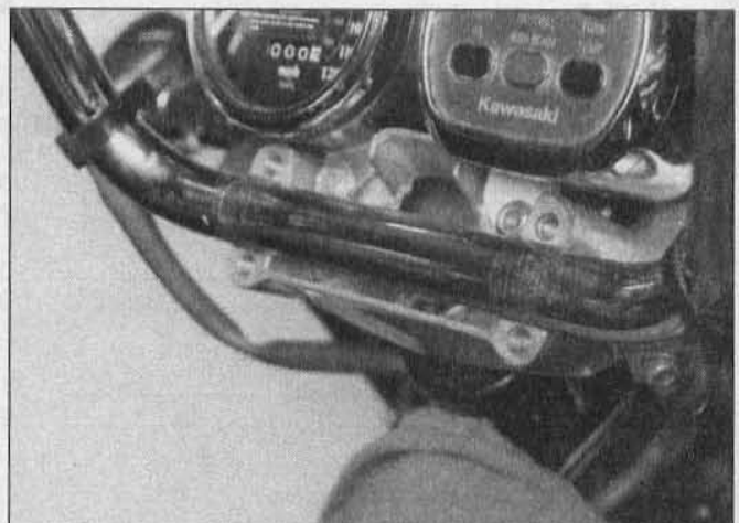
2.1b . . . and lift the handlebar off
