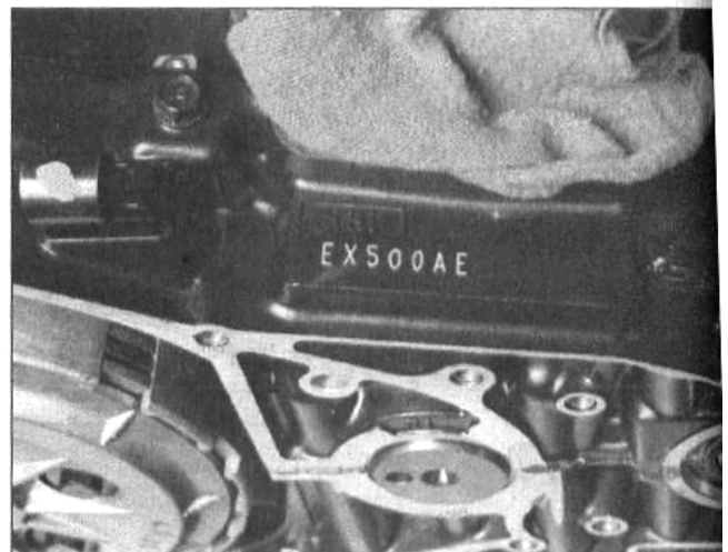
The engine serial number is located on the right side of the engine case
