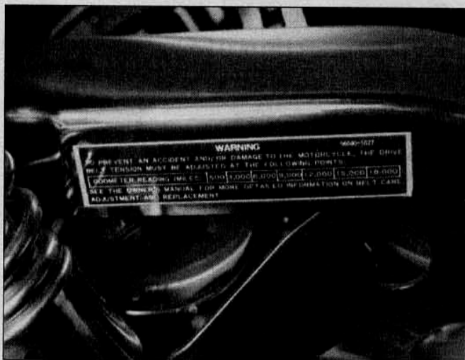
2.3c A decal on the drive belt guard lists belt maintenance intervals
