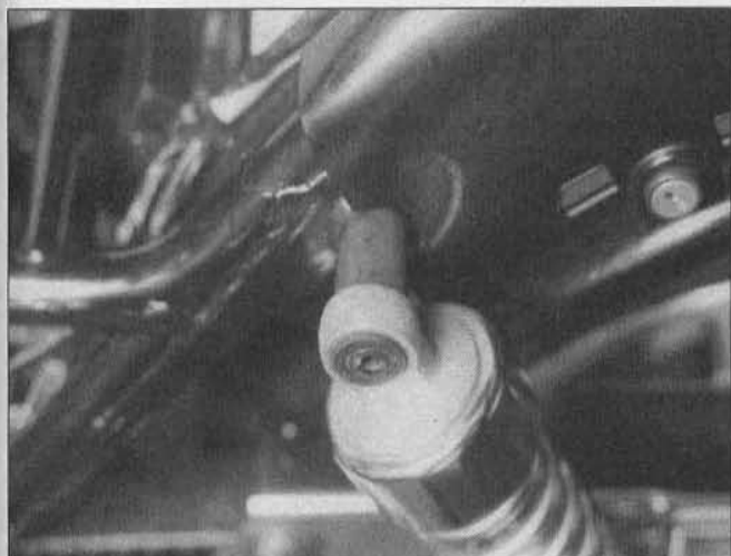
6.3b Once the bolt is removed, the upper end of the shock absorber can be detached from its mounting bracket
