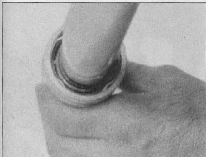
4.21 Install the retaining ring and make sure it seats in its groove
