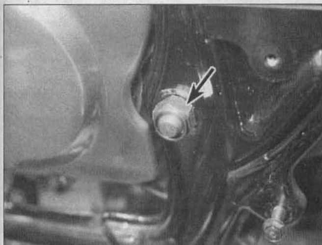
8.5 Remove the swingarm pivot shaft nut and withdraw the shaft
