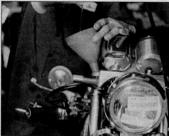
29.7 Use a funnel to pour oil into the fork
