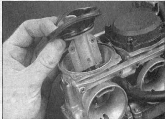
7.4 Remove the diaphragm/piston assembly from the carburetor body
