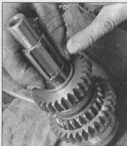
30.15h ...this will expose the bushing shared by third and fourth gears...
