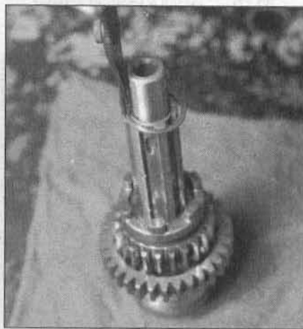
30.17d Install a snap-ring in the groove farthest down the shaft. . .
