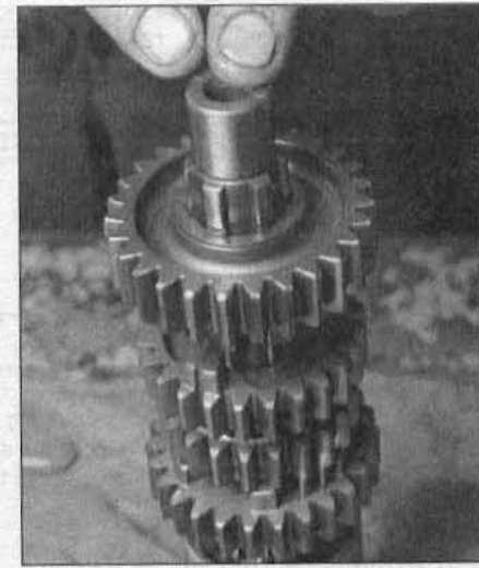
30.11g Install sixth gear with its flat side away from fourth gear and place a toothed washer next to it...
