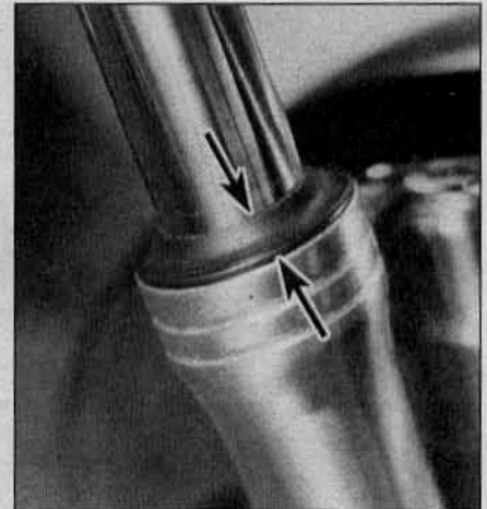
28.3 Check above and below the fork seals (arrows) for signs of oil leakage
